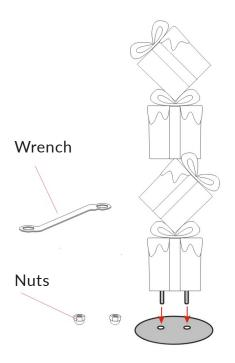
Use your wrench to connect the wire tubes to the metal base with the nuts provided.
