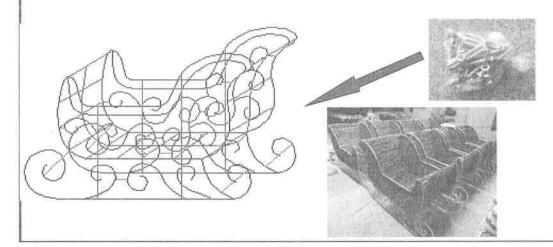
(3) Connect each part of sleigh together with male and female connector, then conenct male connector of side of sleigh, foot of the deer, to power cord, then it will be light up.
