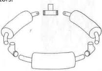
3 Attach 4 loops onto one of the 13" curved pieces. Add a connector marked "TOP" to both ends and repeat with adding 4 more loops onto each of the remaining 13" curved pieces. Insert 6 plastic rivets into each of the pre-drilled holes to secure the base tubes to the connectors.
