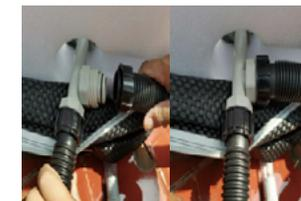
9) Connect the longest connecting hose to the T-joint as shown in the image.
