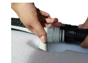
11) Connect the other end of the hose to the two-way connector, as shown in the image.
