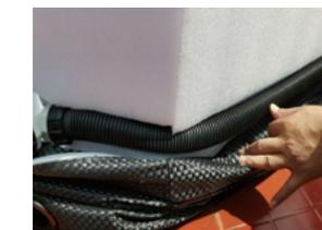
10) Insert the hose into the groove on the foam, as shown in the image.
