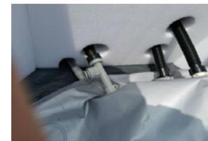
7) Install the connecting hose. (assemble the short hose and the T-joint as shown in the image)
